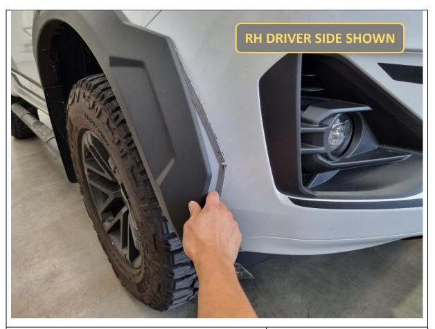
20. Starting from the bottom, pull on the front of the flare and separate it from the bumper.
