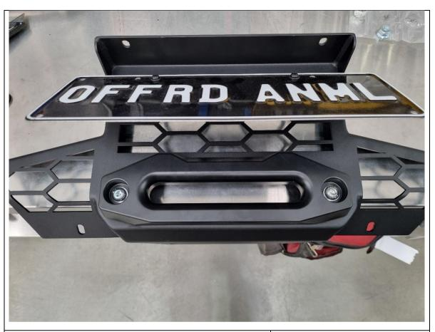
146. If required, fit the winch fairlead to the mesh fairlead mount using M10 or 3/8" fasteners supplied with the winch. This bar is only compatible with hawse type fairleads.
