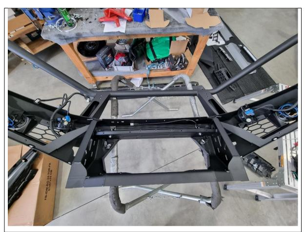
123. Route the fog light bumper wiring harness through the inside of the bullbar.
