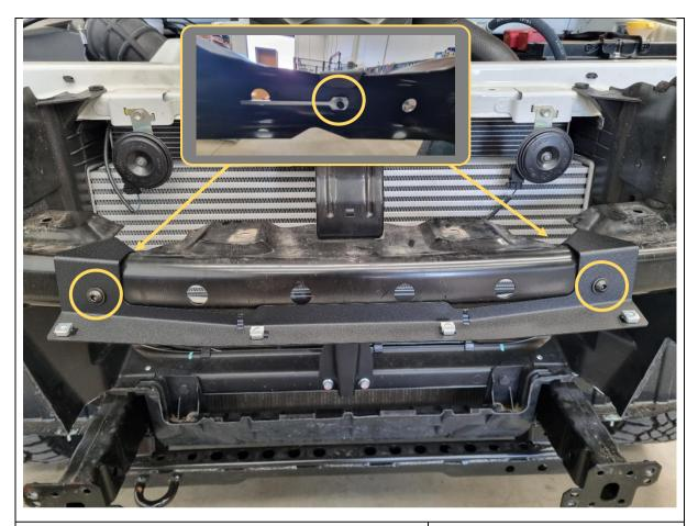
54. Fit the B-1575 grille mount to the vehicle as shown.
