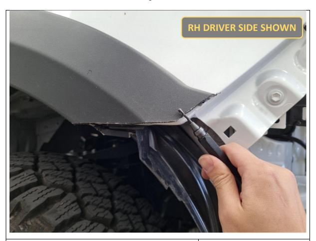
78. Tidy up the flare cut and deburr any sharp edges.
