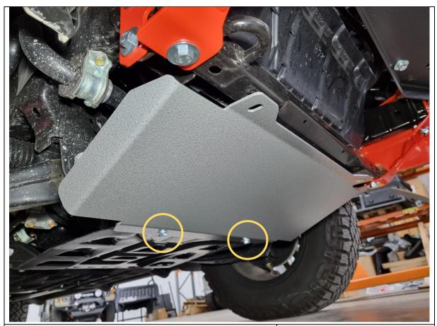
152. Fit the Blade lower bash plate to the vehicle.
