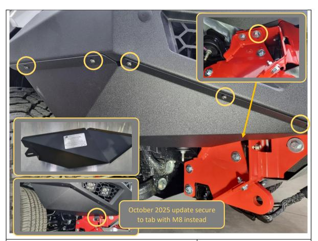
158. Temporarily remove the 2x M10x30 hex bolts from the impact assemblies in preparation for fitting the bash plate. Set them aside.
