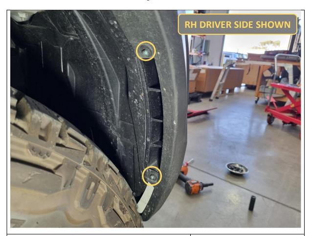
16. In the front wheel well area, remove 2x 8mm hex screws holding the flare to the bumper. Do this for both sides.
