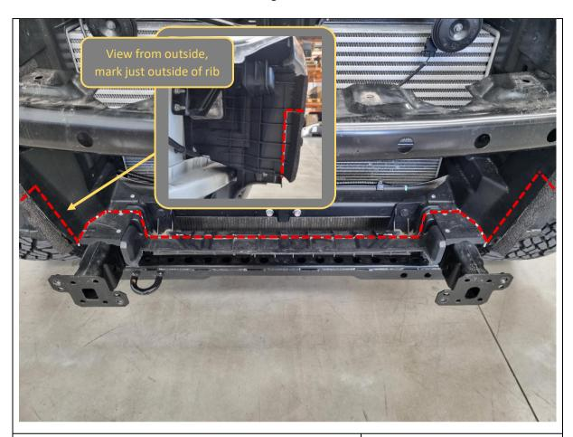
38. The plastic air guide needs to be trimmed. Use a marker pen and mark the air guide using the above images as reference.
