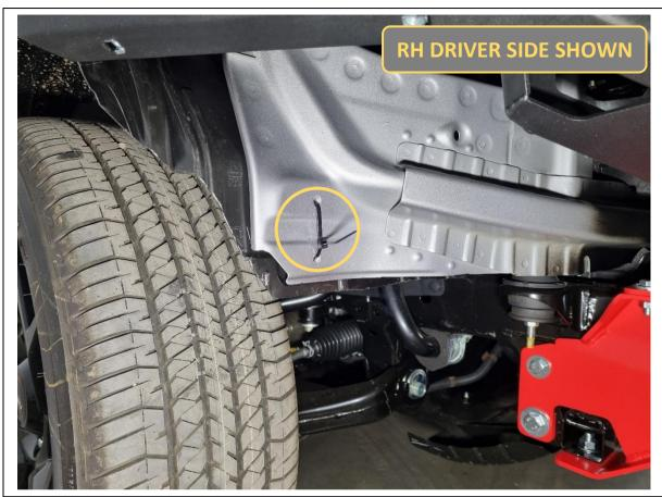
165. **Optional.** Drill a hole through the inner wheel arch liner and use a cable tie to secure it to the body, as shown.
