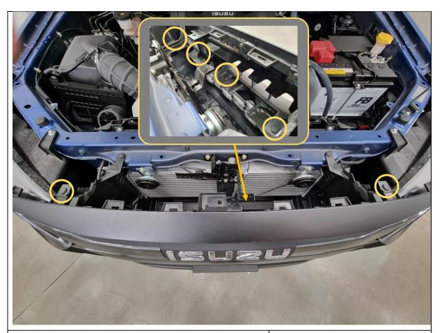
12. Remove 6x plastic push clips holding the grille. There are 2x clips on the top edge, and 4x clips on the cross member on the inside of the grille.
